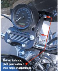
Because of the handlebar clamp-mounted speedometer, the XL883 fitting does not offer as wide a range of adjustment as it does with other Harley models. However, as you can see by the pictures, its adjustability is still quite good. With the Gladiator you can stay warmer, and be cooler.
